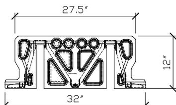
*Cross Section of an Amvic Decking System Form.*
