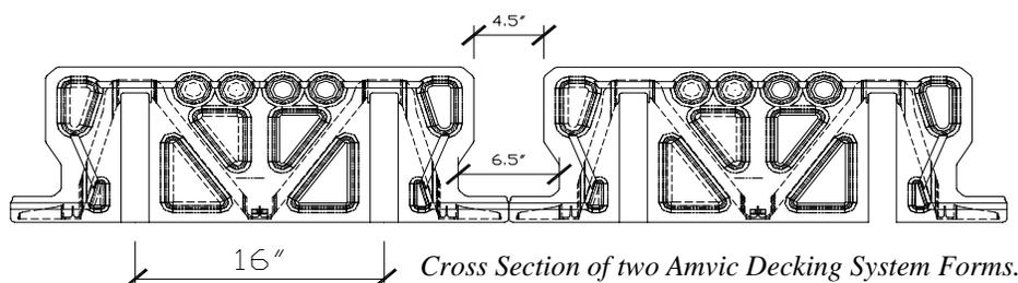
*Cross Section of two Amvic Decking System Forms.*
