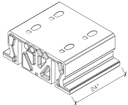
*Isometric view of an Amvic Decking System Form.*
